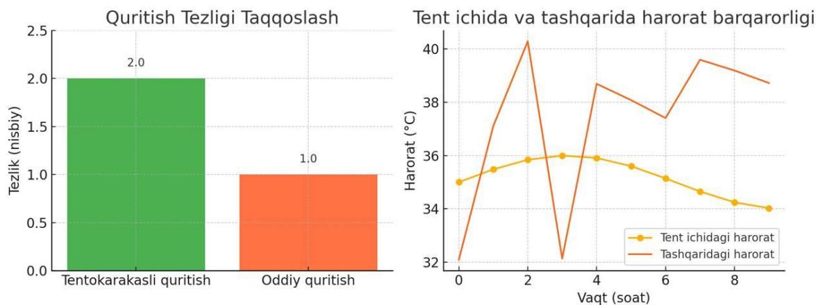
1. **Drying Speed Comparison** — The tent-type method dried products approximately twice as fast as traditional open-air drying.
