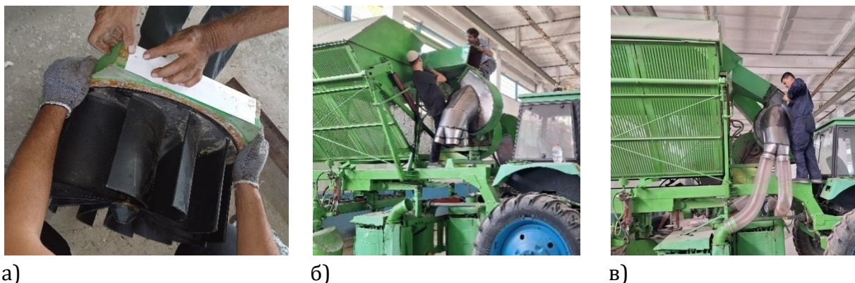
Figure 2. The process of installing an updated fan for air transport system on a cotton picking machine
