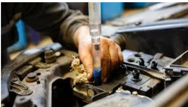
Figure 6. Checking the accumulator batteries
