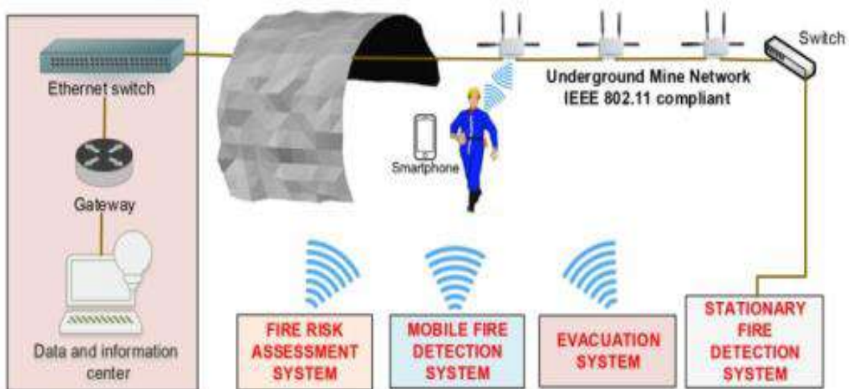
Figure 1. Proposed backbone for underground mine network Prototype Model for Fire Safety System
