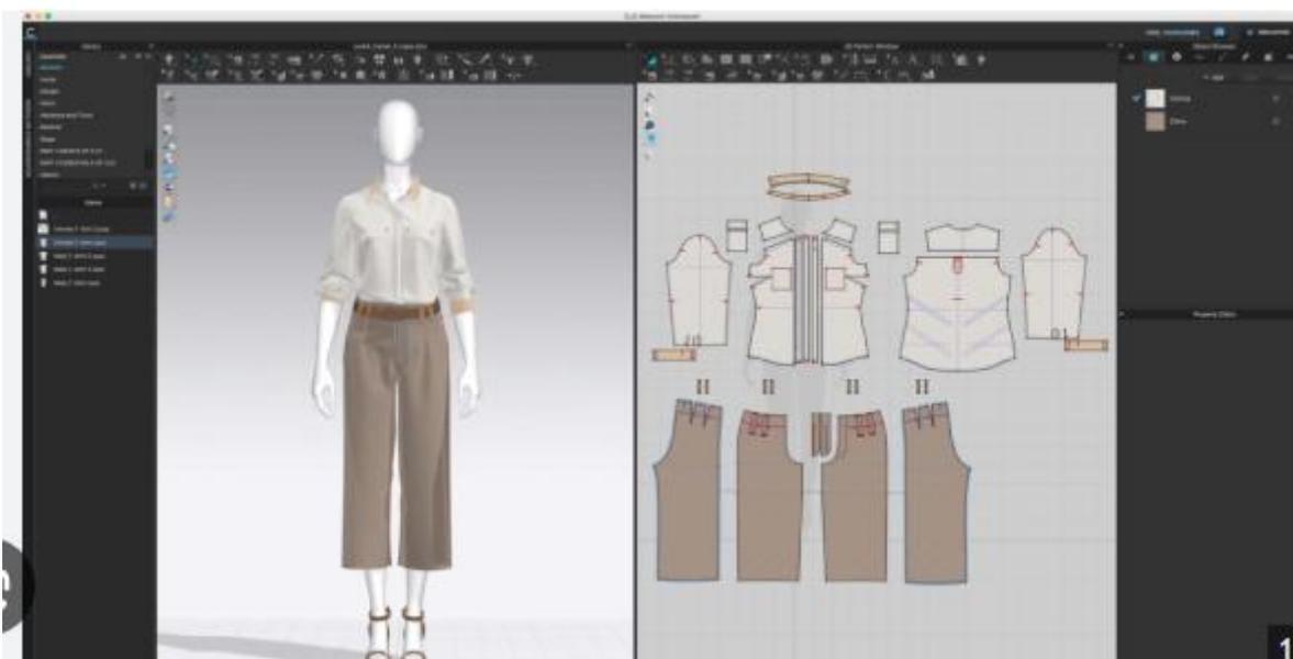
**Figure 3. Garment Design Using CLO 3D**
