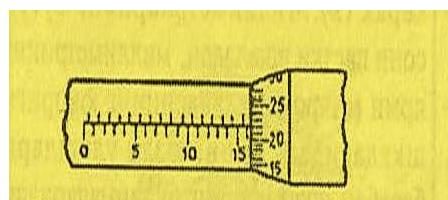
2. Millimeters and half millimeters are counted by the number of divisions in the body of the micrometer bushing. Hundredths of a millimeter is determined by the degree to which the cone of the drum coincides with the longitudinal line of the body.
