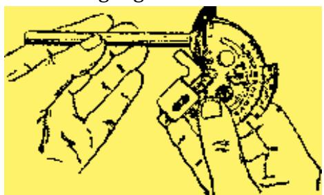
1. The angle measuring sector is set in such a position that the angle between the removable ruler and the edge of the gouge is slightly larger than the measured angle of the part. One edge of the measured angle in the part is placed on the removable ruler of the protractor, the moving ruler is pushed so that the gap between the sides of the measured angle of the part and the burr and the edges of the removable ruler of the protractor is the same be different. The sector is fixed with a stopper.
