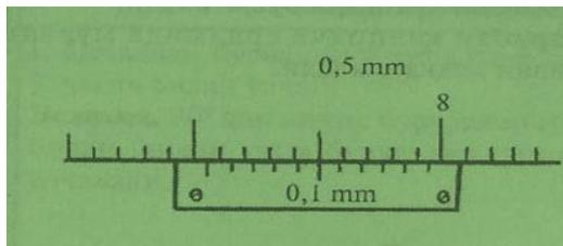
4. The whole number of millimeters is counted to the zero division of the vernier on the bar scale. It is determined that the division of the vernier corresponds to one of the divisions of the barbell. The number of decimal or hundredths of a millimeter is determined by multiplying the number of intervals between the zero division of the vernier and the corresponding division of the bar by the value of the measuring accuracy of the bar circle.
