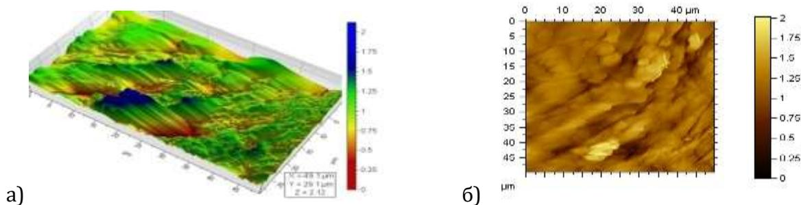
**Figure 2. AFM images of a composite material based on polyamide-66 and basalt: a) - three-dimensional image, b) - two-dimensional image.**
