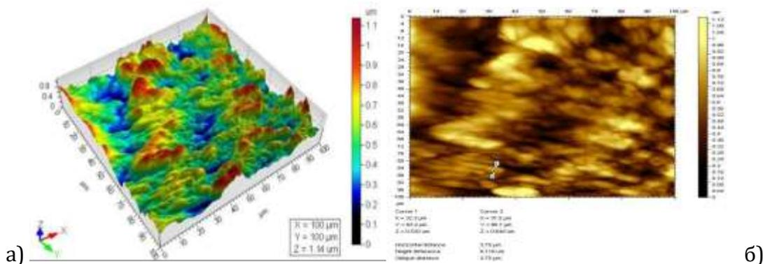
**Figure 1. AFM images of a composite material based on polyethylene with vermiculite a) - three-dimensional image, b) - two-dimensional image.**
